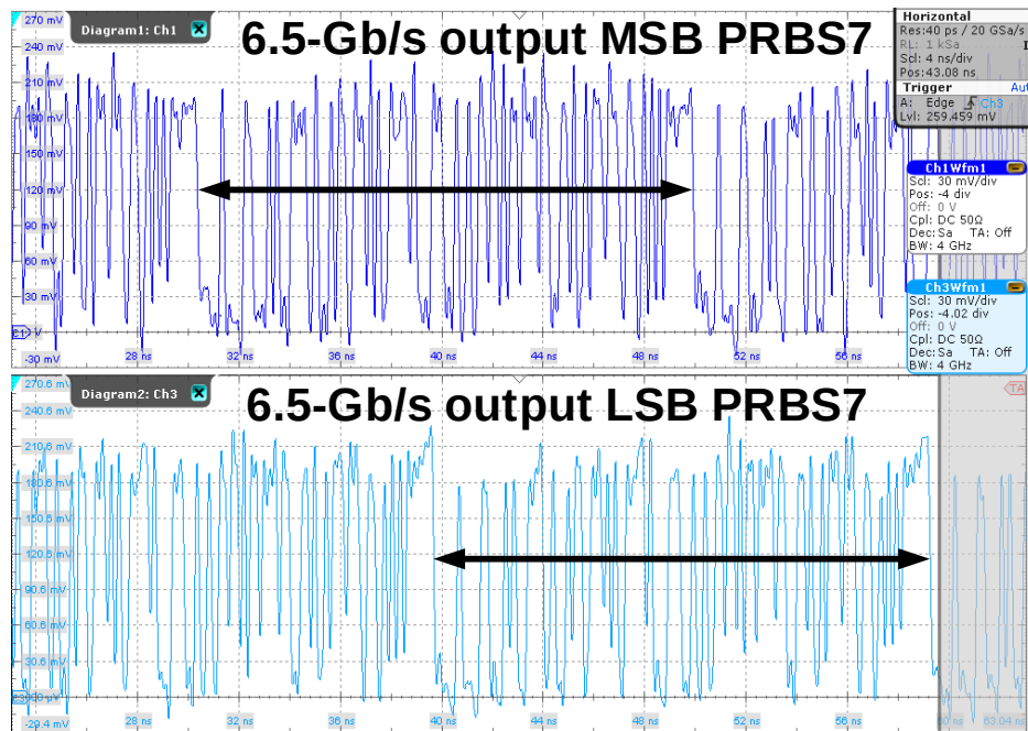
Fig. 40 The decoded PRBS-7 quarter-rate MSB and LSB data transient waveform.
