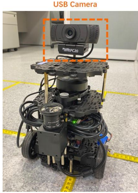
Figure 4.5: The robot equipped with a typical USB camera in the proposed VLP-based image taking robot system.
