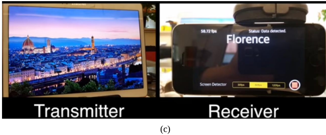
Fig. 1.6 (a) An extra communication layer on top of the content layer, (b) the resulting composite image after modifying the pixel translucency of the communication layer, and (c) demonstration of the system, where the image on the transmitter was encoded with data, and the receiver camera captured the picture to extract the transmitted data, which was displayed on the camera screen [48, 50].
