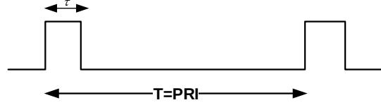
Fig. 2-6. Transmitted pulses with a specified pulse width and PRI.
