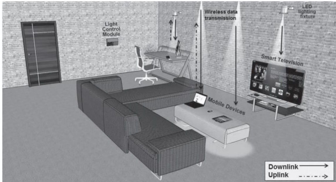
Figure. 1. 4. Application of LED-based optical wireless communication system in indoor environment [13].
