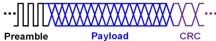
Figure 3.7 VLC Data Packet Format
